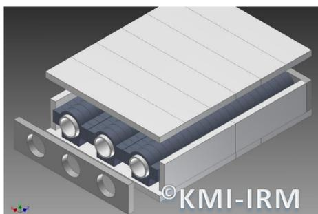
The final design of a section of 3 detector tubes of the second Belgian neutron monitor. It is expected that it will start providing data in 2017 however without the lead-producer.
