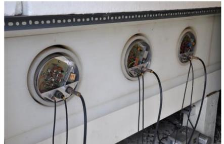
A section of 3 detector tubes from the 9-NM-64 monitor in Dourbes operational from October 1965.
