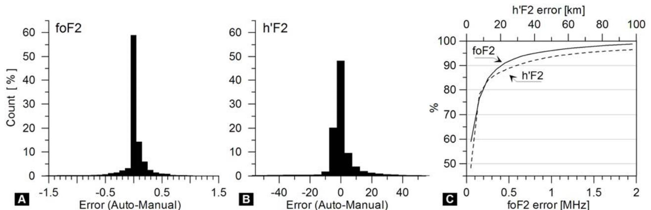
**Fig.1.** Comparison between automatically and manually-scaled ionospheric characteristics for the Dourbes DGS-256 / ARTIST-4 system during the 2002-2008 period. (A/B): Histograms of the foF2 and h'F2 errors. (C): Relative cumulative foF2 and h'F2 error distributions.
