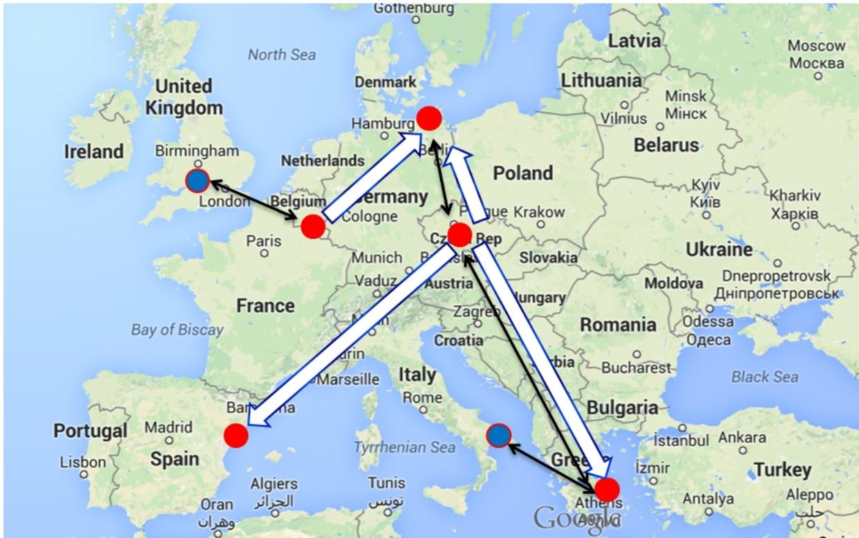
**Figure 1.** DPS4D locations and possible short and long path links under consideration for the pilot network. The DPS4D stations already participating in the project are indicated by the red dots. The NEXION stations are indicated with blue dots. Black arrows denote synchronized vertical and oblique “ionogramming”, white arrows denote Digisonde-to- Digisonde “skymapping”.
