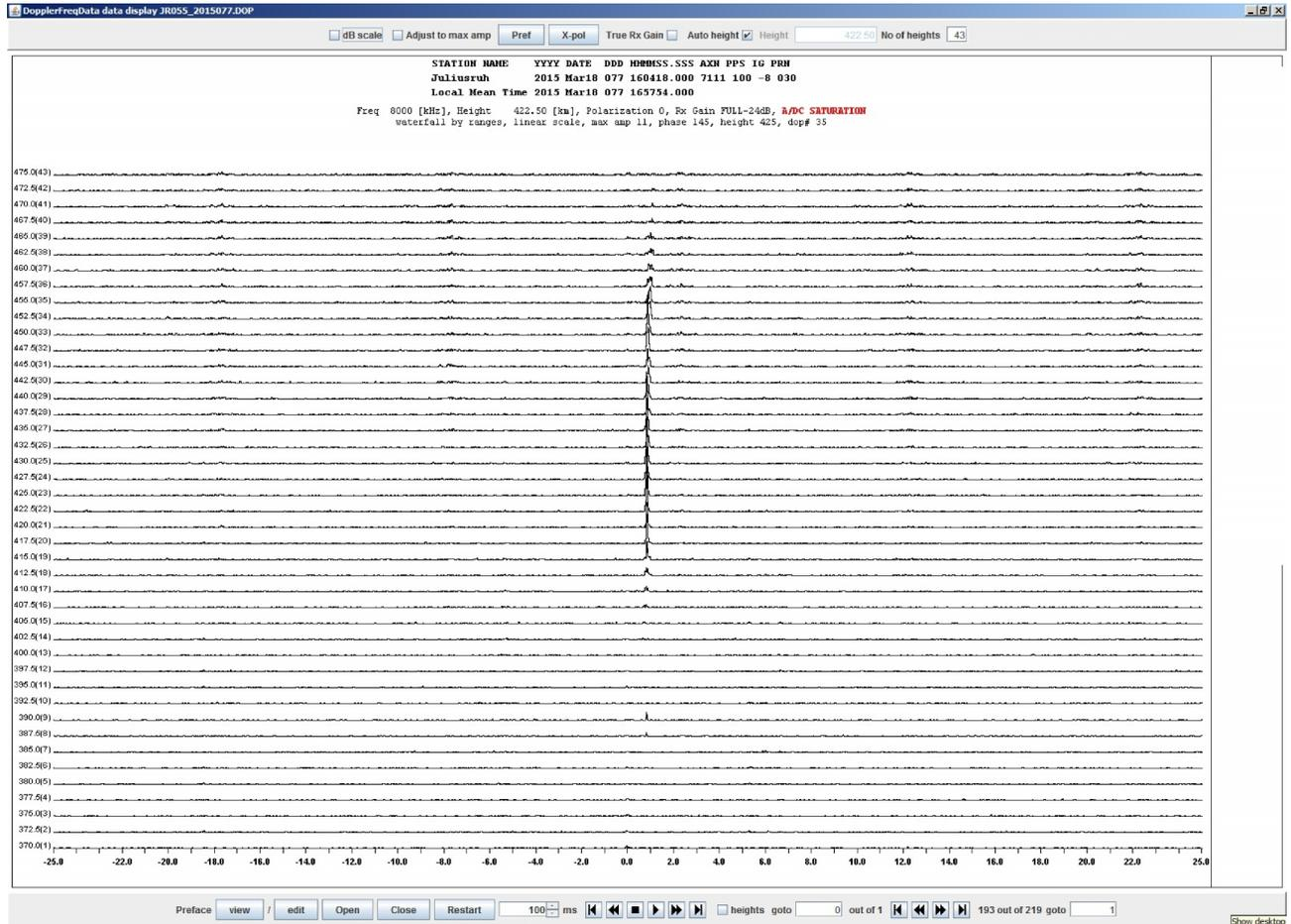
**Figure 3.** D2D waterfall display at Juliusruh listening to the 8.0 MHz transmissions from Pruhonice, recorded on 18 March 2015.
