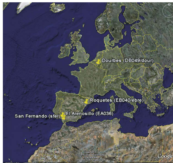
Fig. 1. Collocated digisondes and IGS/EUREF stations.
