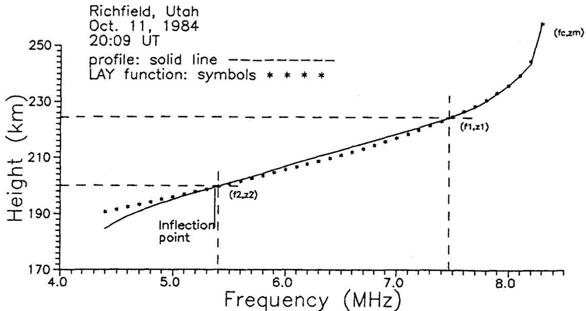
Figure 1. Fitting LAY function profile. The three selected points were (8.3 MHz, 285 km), (7.5 MHz, 224 km), and (5.4 MHz, 200 km). The LAY function approximates the F2 profile to frequencies well below the inflection point. foF1 for this ionogram is 4.3 MHz.
