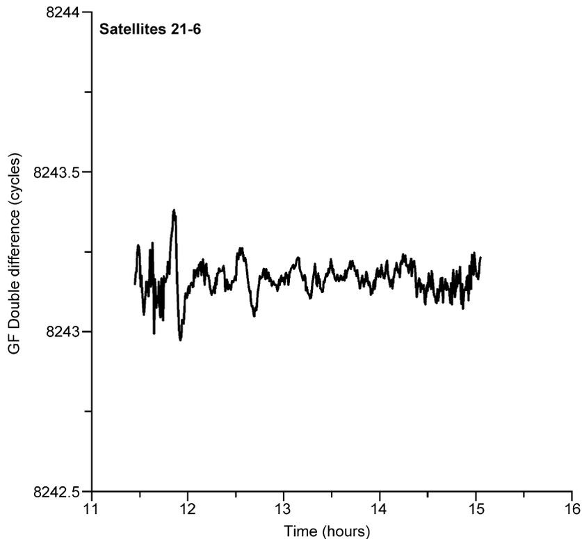
Fig. 7. Double difference of the geometric free combination on DOY 359 in 2004, baseline Brussels–Saint-Gilles, satellite pair 21-6.
