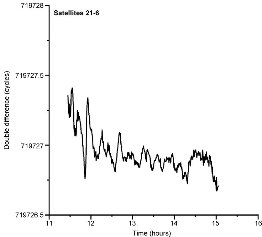
Fig. 8. Double difference of the L1 phase on DOY 359 in 2004, baseline Brussels–Saint-Gilles, satellite pair 21-6.
