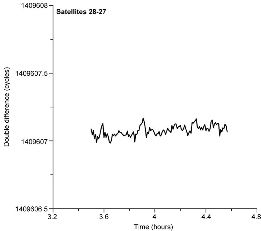
Fig. 5. Double difference of the L1 phase on DOY 359 in 2004, baseline Brussels–Saint-Gilles, satellite pair 28-27.
