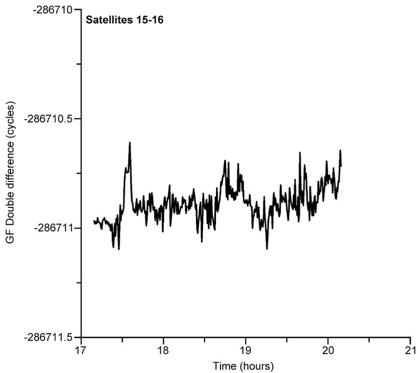
Fig. 11. Double difference of the geometric free combination on DOY 324 in 2003, baseline Brussels–Saint-Gilles, satellite pair 15-16.
