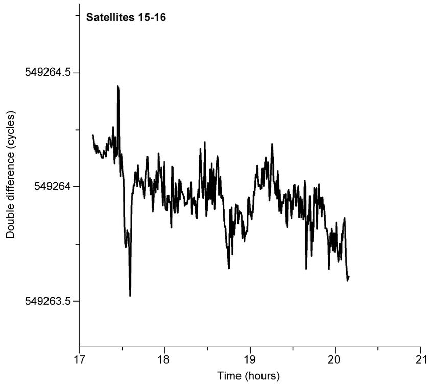
Fig. 10. Double difference of the L1 phase on DOY 324 in 2003, baseline Brussels–Saint-Gilles, satellite pair 15-16.
