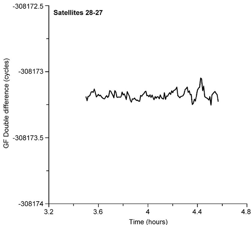
Fig. 4. Double difference of the geometric free combination on DOY 359 in 2004, baseline Brussels–Saint-Gilles, satellite pair 28–27.
