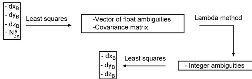
Fig. 3. Algorithm of our RTK simulation software
