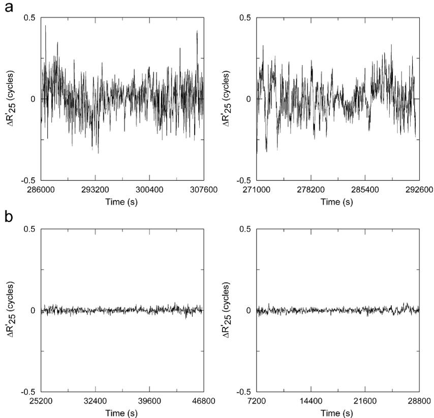
Fig. 1. Influence of code multipath delays and code measurement noise on the EWL ambiguities  $N_{25}$  ( $\Delta R_{25}$ ) for two GPS (a) and Galileo (b) satellites.
