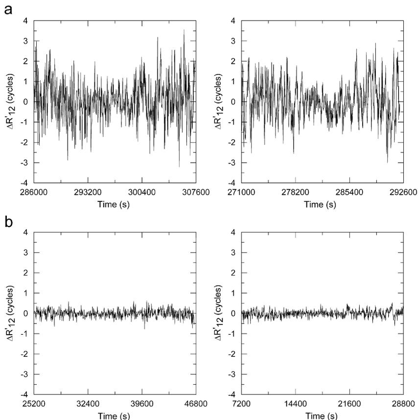
Fig. 2. Influence of code multipath delays and code measurement noise on the WL ambiguities  $N_{12}$  ( $\Delta R_{12}$ ) for two GPS (a) and Galileo (b) satellites.
