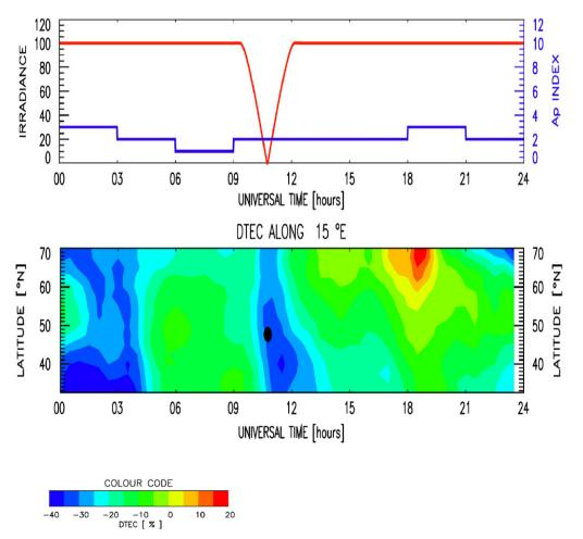
Fig. 16. Diurnal variations of the differential TEC (%) on 11 August 1999 within the latitudinal range from  $30^{\circ}$ N to  $70^{\circ}$ N along the  $15^{\circ}$ E meridian. The corresponding obscuration function is plotted in the top panel.
