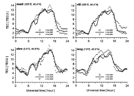
Fig. 9. Comparison of TEC measurements at different GPS stations, carried out on 2–4 October 2005 at different GPS receiver stations in Spain. Notice the significant plasma loss of 20–30% during the eclipse on 3 October 2005.
