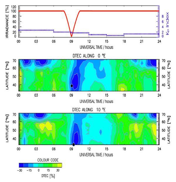
Fig. 11. Diurnal variations of the differential TEC (%) on 3 October 2005 within the latitudinal range from  $30^{\circ}$ N to  $70^{\circ}$ N along the  $0^{\circ}$ E (middle panel) and  $15^{\circ}$ E (bottom panel) meridians. The obscuration function is plotted for  $0^{\circ}$ E in the top panel.
