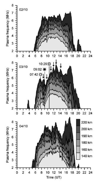
Fig. 5. Diurnal variations of plasma frequency at fixed "true" heights at Ebro observatory ( $40.8^{\circ}$ N,  $0.5^{\circ}$ E). The moments of the start, maximum occultation, and end of solar eclipse (as seen at ground level) are clearly indicated on the plot of 3 October 2005. The wave crests are marked with arrows.
