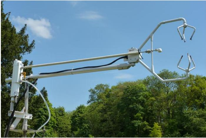
Figure 29: Installation of the eddy-covariance system at Uccle in 2018.
