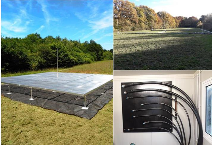
*Figure 32: The future transmitter of the meteor radar (left), the five antennas of the interferometer of the meteor radar (top right), and the RF coaxial cables inside the container (bottom right).*
