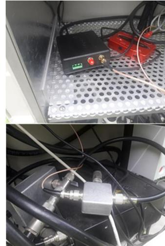
*Figure 34: The RSP2 receiver and the external sound-card used by the current system to sample the signal going out of the ICOM-R75 receiver (Top). The power splitter used to split the incoming signal from the antenna between the ICOM-R75 and the RSP2 receivers (Bottom). Pictures were taken at the BEUCCL station.*
