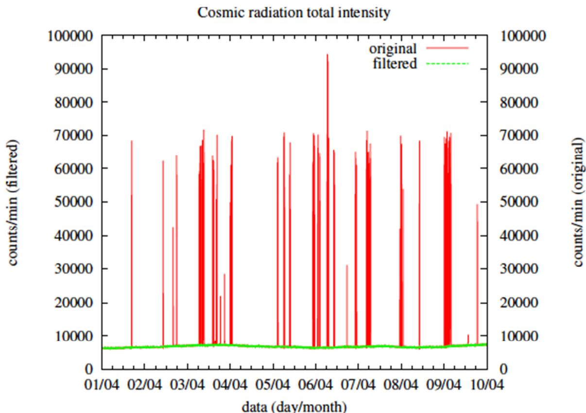
Fig.4-1: Original uncorrected and unfiltered cosmic radiation intensity measurements: counts from individual noisy tubes (in this case, tube 4 and, occasionally, tube 2 and 3 simultaneously) produce very large peaks in the total intensity. The data has been filtered and plotted (dashed line) in the same figure for comparison.
