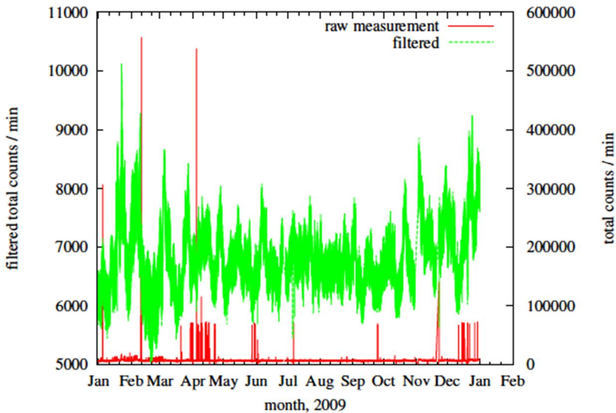
Fig.4-4: An example of single high-intensity peaks at different time intervals being removed by the median filter. Note that these peaks differ from the noisy data displayed in Fig.4-1 in that they come from simultaneous noisy values from all sections of the station while the peaks in Fig.4-1 occur as a result of a limited number (not more than) four erroneous sections (data from 2009).
