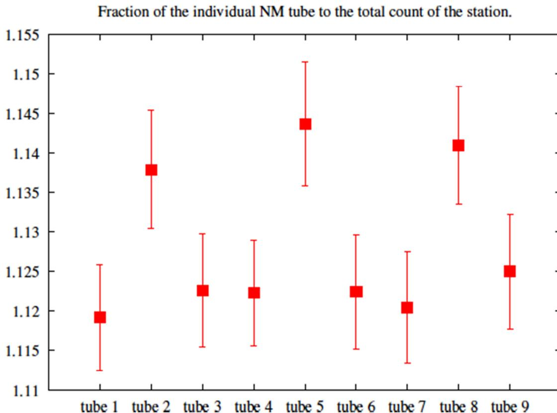
Fig.4-2: Tube factors for correcting the total count rate for a faulty reading. The larger factors (tubes #2, #5, and #8) are (probably) due to the fact that these tubes are newer or with different characteristics (see text).
