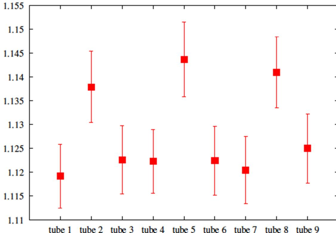
Fig.4-2: Tube factors for correcting the total count rate for a faulty reading. The larger factors (tubes #2, #5, and #8) are (probably) due to the fact that these tubes are newer or with different characteristics (see text).
