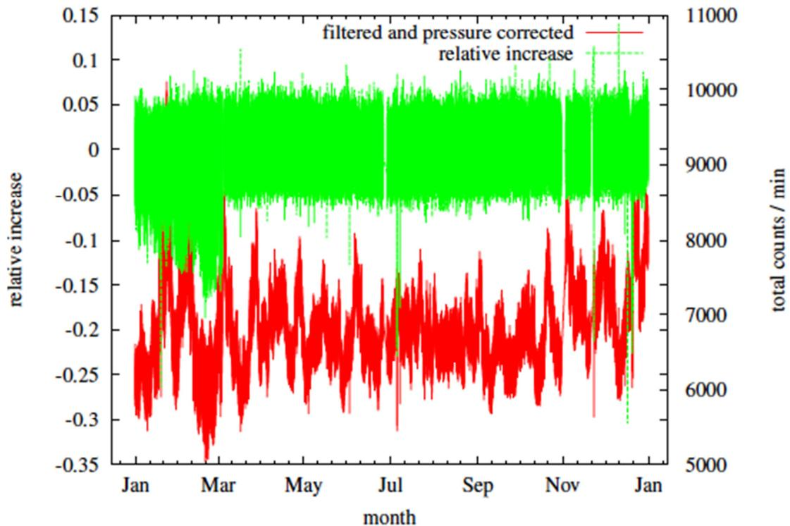
Fig.4-6: Filtered and pressure corrected cosmic ray intensity measurements at Dourbes from year 2009. This data is used to obtain the baseline reference intensity for the station which in turn is used to calculate the relative intensity increase. The latter is the reported data which is also used for detection of solar effects on the intensity of the galactic cosmic rays.
