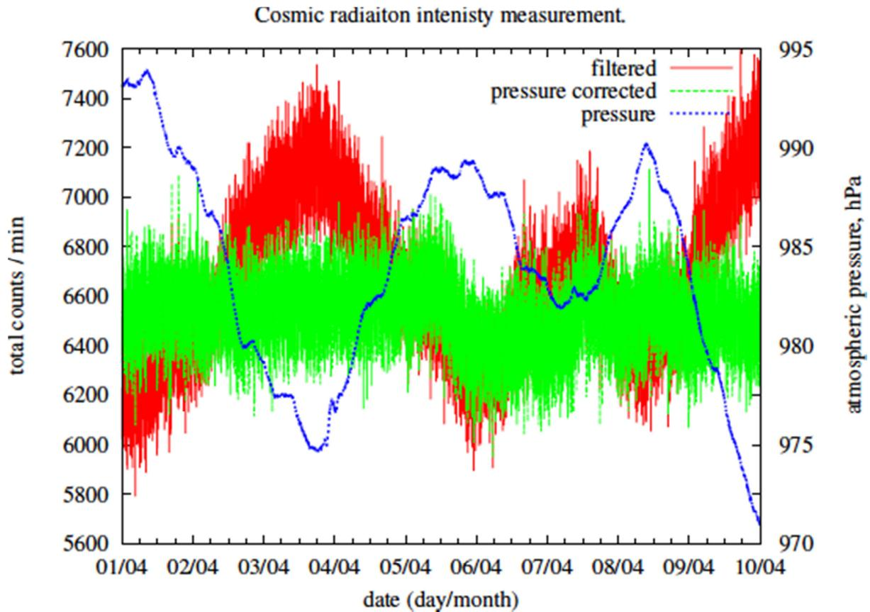
Fig.4-3: Filtered cosmic radiation intensity, plotted together with the atmospheric pressure and the same data corrected for pressure.
